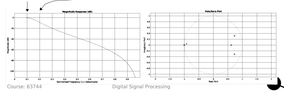
• How we can map continuous-time filters to discrete-time domain?  $\rightarrow$  transformation  $H_c(s) \rightarrow H(z)$ ,  $s = \sigma + j\Omega$ , where  $\Omega$  is the analog frequency
