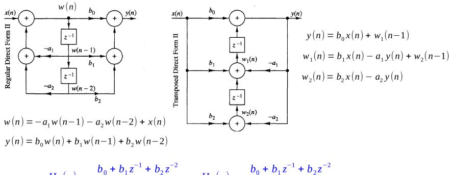
$$H_{\rm II}(z) = \frac{b_0 + b_1 z^{-1} + b_2 z^{-2}}{1 + a_1 z^{-1} + a_2 z^{-2}} = H_{\rm T}(z) = \frac{b_0 + b_1 z^{-1} + b_2 z^{-2}}{1 + a_1 z^{-1} + a_2 z^{-2}}$$
